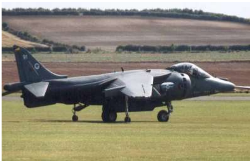
Monotrace Landing gear of a Harrier fighter jet.
