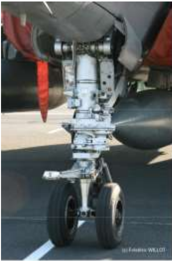
Twin wheels Nose gear of a Rafale
